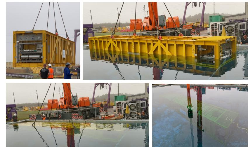
Figure 2. A dry factory acceptance test (FAT) was completed, followed by a system integration test (SIT).
