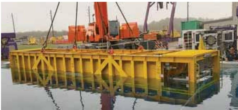
A prototype of a chemical delivery unit lifted and then lowered into a test pool in Katy, Texas. *Source: Safe Marine Transfer.*
